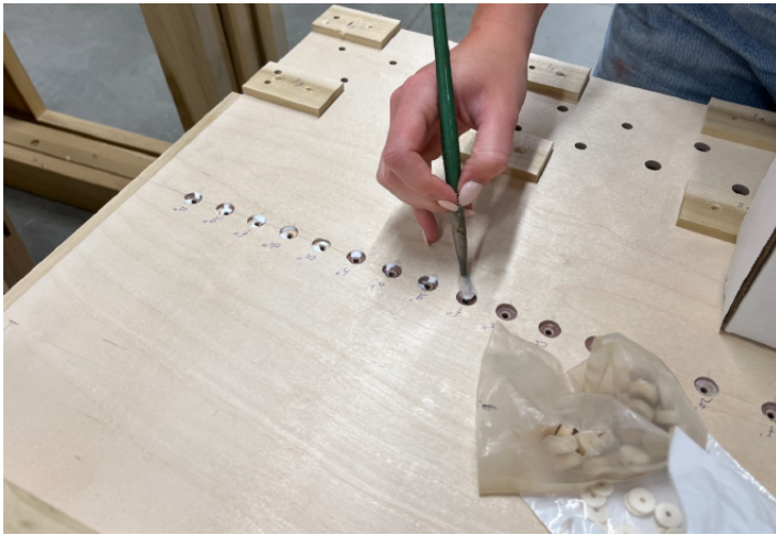
Glueing felt into the bleeder holes of the windchests.
