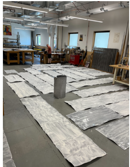
Steven laying out the lead sheets that will be used for the facade
