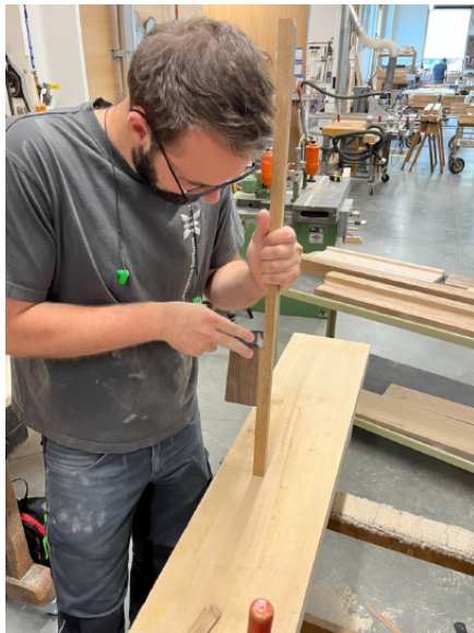
David working on the sharps of the pedal board.
