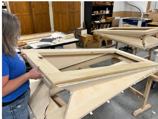
Maurine gluing the tabs onto the belows.
