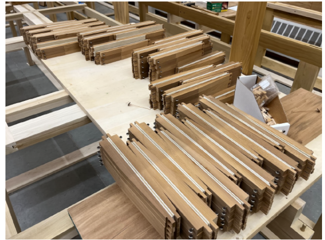
Completed pallets ready to be placed in the windchests.
